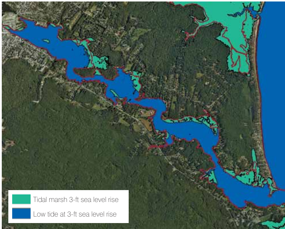
FIGURE 3 Projected 3-ft sea level rise by 2100 in the Saco Estuary. Green areas are predicted future areas of tidal marsh. The blue area is the low tide water level, and the red line is the 2011–2012. Highest Annual Tide (HAT) line.
