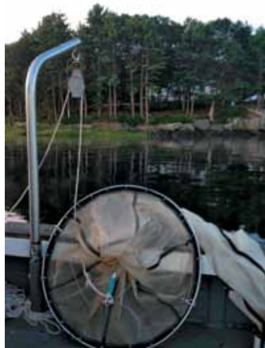
FIGURE 4 Plankton tow net used to collect larval fish at multiple locations within the Saco estuary.
